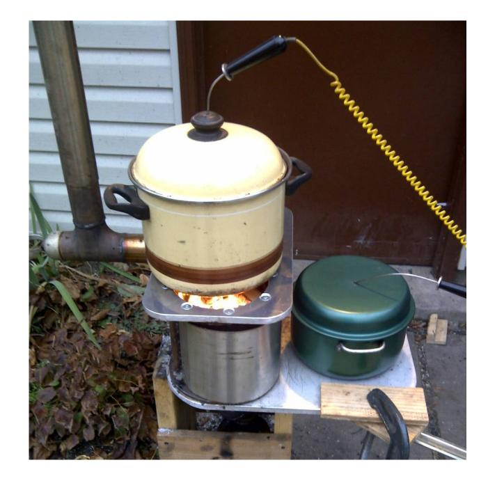
Reflective stainless steel cowl constrains radiative and convective losses, forcing more heat into the conductive plates.
